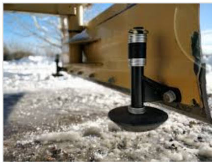
Figure 5: Common plow blade skids.
