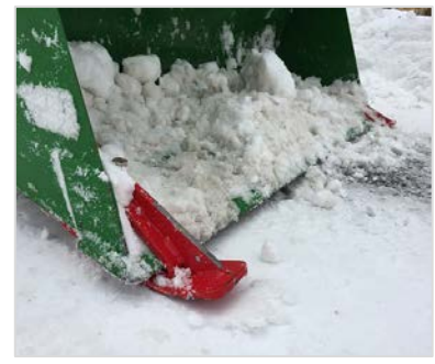
Figure 6: Sled-type skid attachments.
