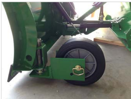
Figure 4: Skid roller attachments.
